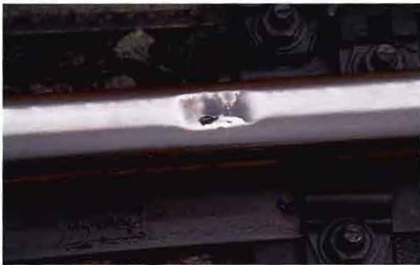
*Experimental study of cracks in rails caused by rolling contact fatigue*
