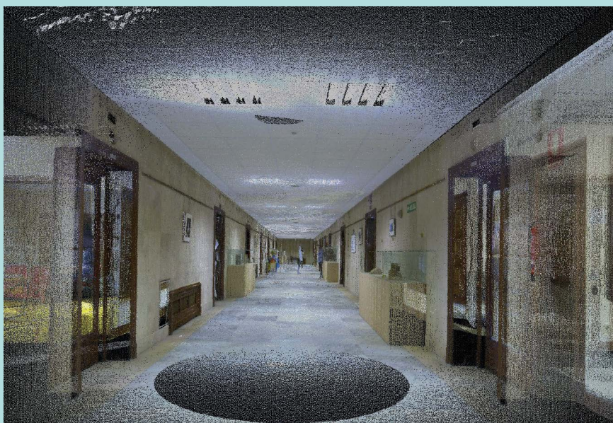
Point cloud of a corridor in the Ministry.
